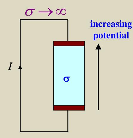
• The current / must be zero since the electrons cannot gain back the energy they lose in traveling through the resistor.
