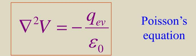
$\Rightarrow \nabla^2$  is the *Laplacian operator*. The *Laplacian* of a scalar function is a scalar function equal to the divergence of the gradient of the original scalar function.
