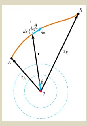
Consider isolated positive point charge q. (i.e. E directed radially outward from the charge)
