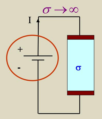
To maintain a steady current, there must be an element in the circuit wherein the potential <u>rises</u> along the direction of the current.
