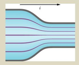
The concept of streamlines: stream lines that are closer together imply greater current density.
