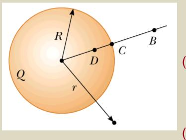
An insulating solid sphere of radius R has a uniform positive volume charge density and total charge Q.
