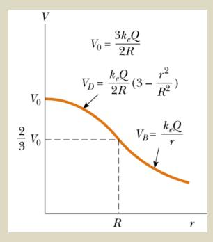
What are the magnitude of the electric field and the electric potential at the center of the sphere?
