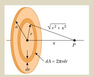
(a) Find an expression for the electric potential at point P located on the perpendicular central axis of a uniformly charged disk of radius a and surface charge density  $\sigma$ . (b) Find an expression for the magnitude of the electric field at point P.
