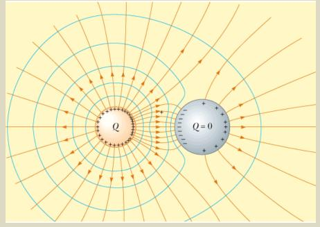
The electric field lines (in orange) around two spherical conductors. The smaller sphere has a net charge Q, and the larger one has zero net charge. The blue curves are cross sections of equipotential surfaces.
