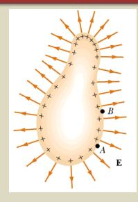
An arbitrarily shaped conductor carrying a positive charge. When the conductor is in electrostatic equilibrium, all of the charge resides at the surface, E = 0 inside the conductor, and the direction of E just outside the conductor is perpendicular to the surface. The electric potential is constant inside the conductor and is equal to the potential at the surface.
