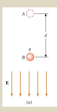
If  $q_o$  is positive then DU is negative. i.e. a positive charge loses electric potential energy when it moves in the direction of the electric field.
