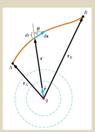
$$V_{B}-V_{A} = -\int_{A}^{B} E_{r} dr = -\int_{r_{A}}^{r_{B}} kq/r^{2} dr$$
