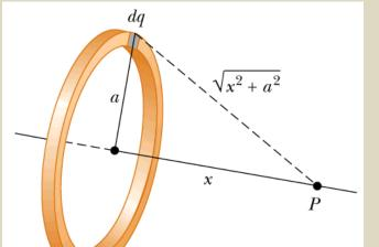
(a) Find an expression for the electric potential at point *P* located on the perpendicular central axis of a uniformly charged ring of radius *a* and total charge Q. (b) Find an expression for the magnitude of the electric field at point P.
