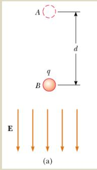
If  $q_o$  is negative then DU is positive and the situation is reversed: a negative charge gains electric potential energy when it moves in the direction of the electric field.
