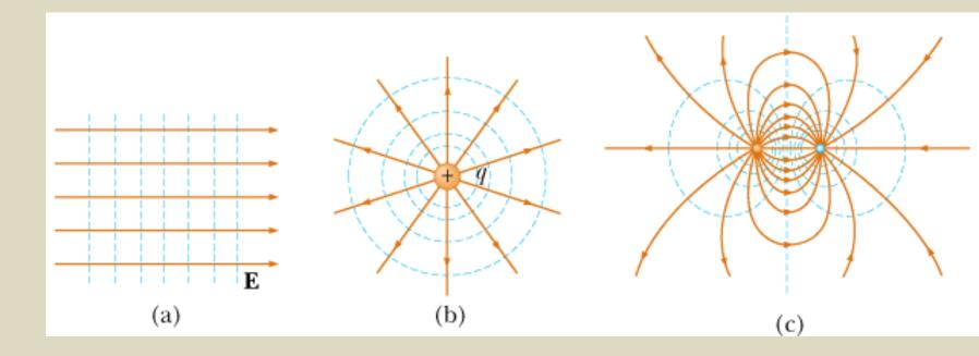
Equipotential Surfaces (dashed blue lines) and electric field lines (orange lines) for (a) a uniform electric field produced by infinite sheet of charge, (b) a point charge, and (c) an electric dipole. In all cases, the equipotential surfaces are perpendicular to the electric field lines at every point.
